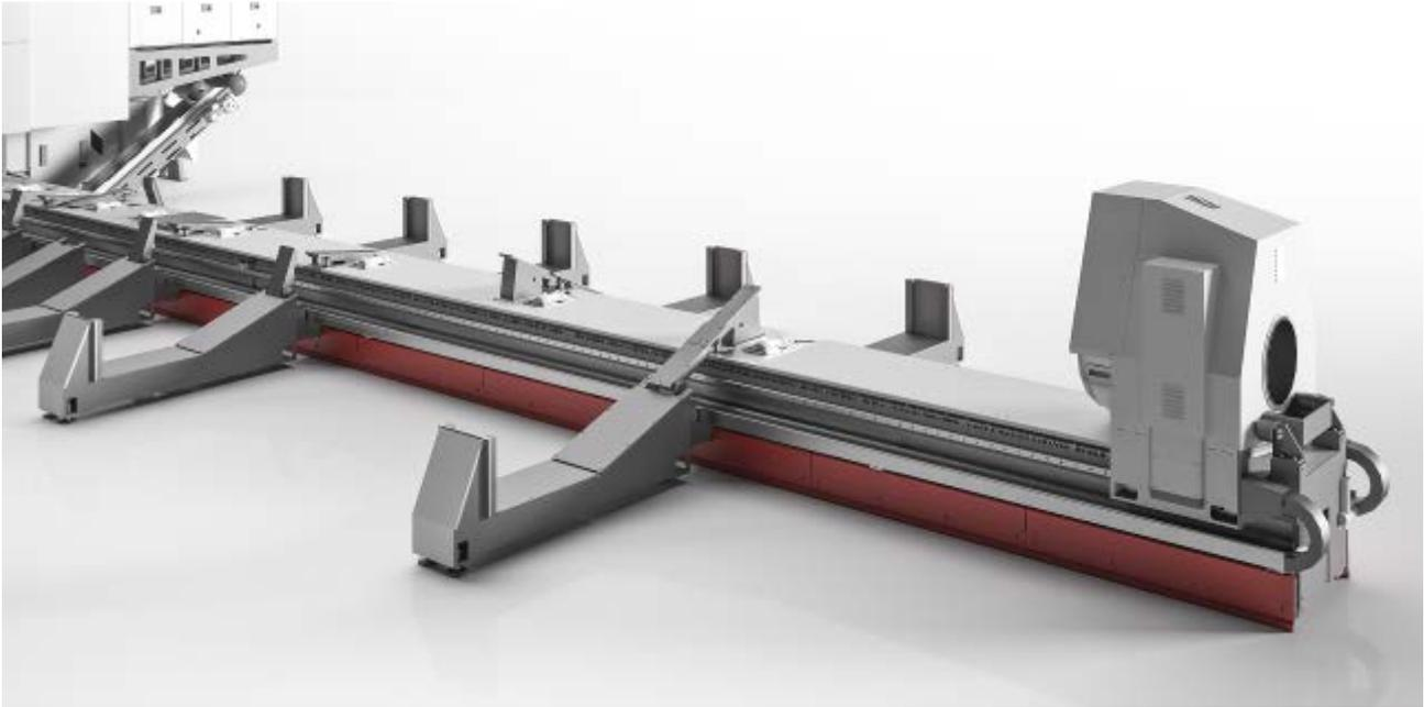
The first and the third mandrel (chuck) (M1 and M3) are expected to clamp the tube ends.
