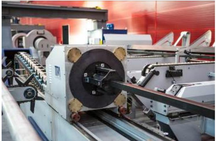
The first mandrel/chuck (M1) is expected to clamp the tube ends by means of jaws. The second mandrel/chuck (M2) fixes the tube near the cutting area and allows the transfer of the tube to the cutting area by means of idle rollers positioned directly on the jaws. M2 as well as M1 is equipped with four sliding and self-centring jaws, activated by pneumatic cylinders and synchronized two by two.
