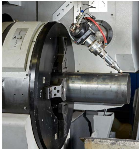
Through a sensor, it is possible to keep the exact focusing distance from the surface to cut. Furthermore, thanks to this sensor, any eventual collisions between the head and scraps or other parts are avoided.
